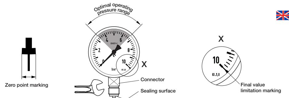
The tapping points should be prepared according to the indications for tapped holes. Further information you will find in the VDE/VDI directive 3511 and 3512 page 3 and EN 837-1/2.
